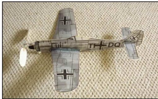
FW 190 6.15g plus 0.57g to balance. Rubber 0.070", has a motor stick of 2 pieces of firm 1/16 x 1/4 glued in an "L" shape and is plenty rigid enough for the rubber sizes we are talking about. Paul Bradley design, printed tissue finish, has done circa 1 minute at Berinsfield by bouncing along the ceiling. [Photo: Dave King].
