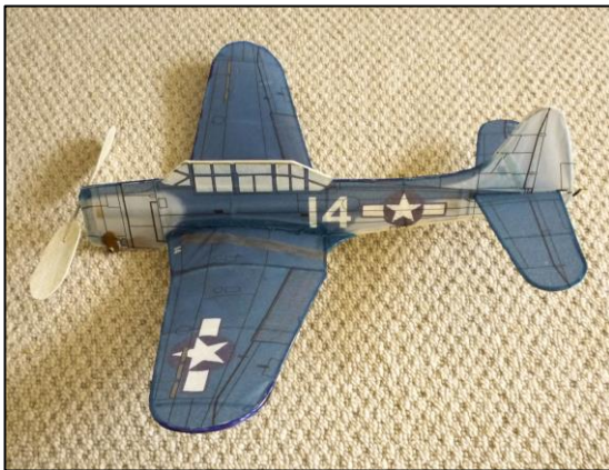
Dauntless 8.30g plus 1.03g weight to balance motor. Rubber 0.080", has a rolled 1/32 tube motor stick but I don't see any advantage over the one used on the FW190. Paul Bradley design, printed tissue finish, trimming still in progress. [Photo: Dave King].
